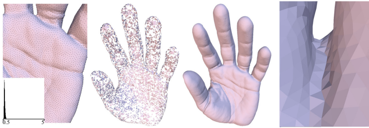
Fig. 10. We consider the Oliver hand model. We see from the left figure that the hand has very uniform sampling. The two hands in the middle show the reconstruction using using k = 3 with 10% correct (left) and k = 7 with 100% correct (right). Notice from the most right figure that the regions between the fingers with high curvature are reconstructed properly.
