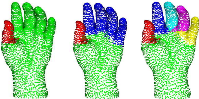
Figure 5. Three levels in the hierarchical segmentation of hand model. The figure on left shows the first bisection of hand that segments out the thumb. The middle figure shows the second bisection where the rest of fingers are segmented out from the palm. The figure on right show the sixth and the last bisection where each fingers have been segmented out.
