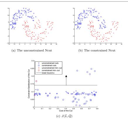
Fig. 4 The joint numerical range of the normalized graph Laplacian  $\bar{L}$  and the normalized constraint matrix  $\bar{Q}$ , as well as the optimal solutions to unconstrained/constrained spectral clustering.
