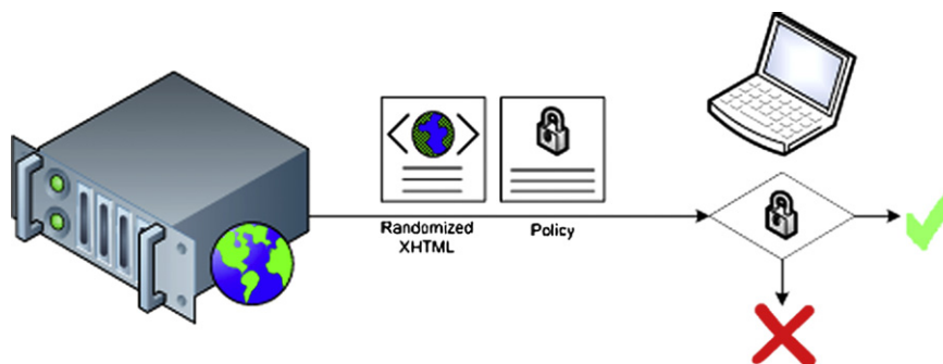
Fig. 2 – Noncespaces overview. The server delivers an (X)HTML document annotated with trust class information and a policy to the client. The client accepts the document only if it satisfies the policy.
