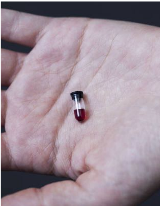
A 'nanotainer' developed by Theranos to help it run tests from just a few drops of blood pricked from a person's finger. The tiny tube is about half an inch long. PHOTO: MARTIN E. KLIMEK
