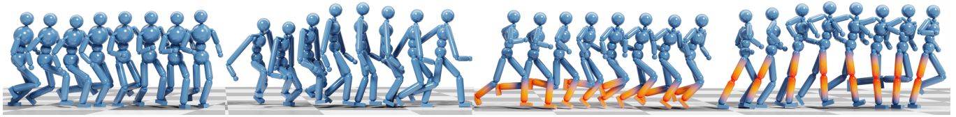
Fig. 9. Adapting the locomotion policy of running to characters with different body shapes and locked joints.
