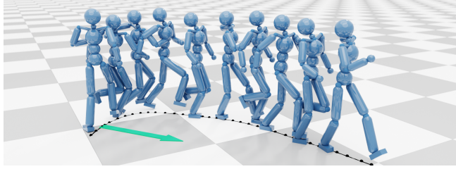
Fig. 5. Example of motion style transfer learning with goal-steering navigation using AdaptNet. Green arrow indicates the dynamically generated target directions for locomotion control.
