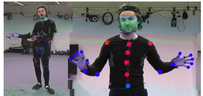
Fig. 3. Capture setup and location of joints. The 16 red markings indicate the joints used for the gesture phase classification. The five green markings indicate the spinal joints added to the joint set for gesture motion prediction.
