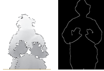
Figure 1. Edge extraction. (Left) Grayscale image before edge extraction. (Right) Result.
