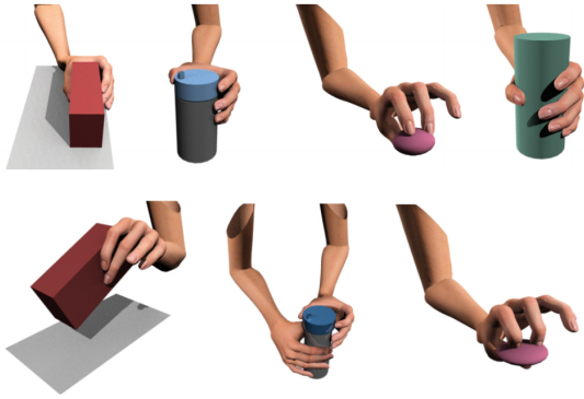
Figure 9: Examples of input grasp poses (top) and poses modified to perform manipulations (bottom) in the physics-based method proposed by Liu [Liu09].
