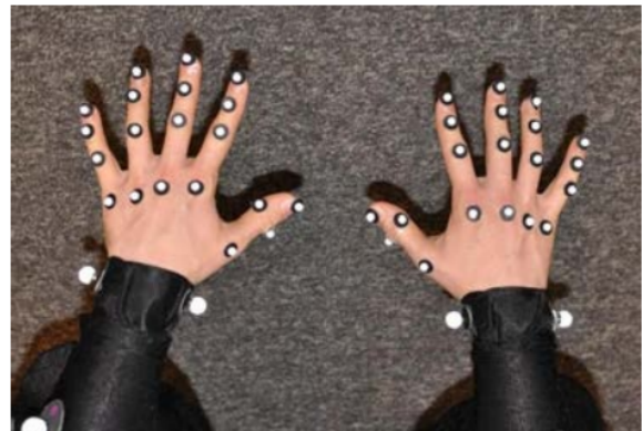
Figure 5: Hands outfitted with a fairly comprehensive marker set for optical motion capture. Further markers could be added to capture the motion of additional joints such as the CMC joint.
