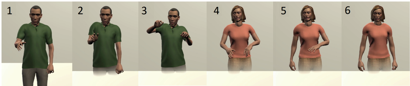
Figure 1: Sample frames from the experiment. (1) The male character in the FK condition, and (2) the same frame in the IK condition and (3) in the IK full error condition where hand tracking was lost for the character's right hand which subsequently remains hanging at shoulder height. (4) The female character in the IK hybrid condition: When tracking for the hand is lost around waist height (character's right hand), the hand will be moved to a rest position. (5) The character's right hand moved to a rest position. (6) Both hands moved to a rest position.
