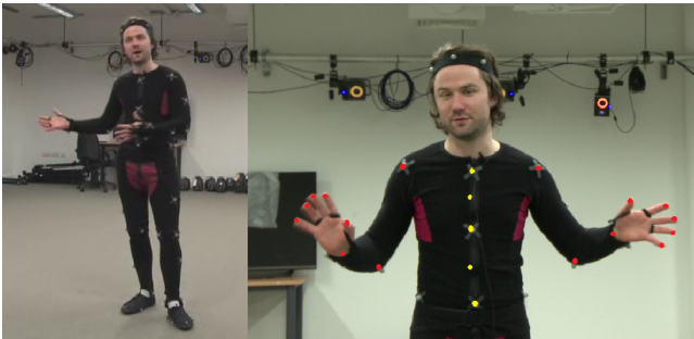
Figure 2: Capture setup and location of joints. The 16 red markings indicate the joints used for the gesture phase classification. The five yellow markings indicate the spinal joints added to the joint set for gesture motion prediction.
