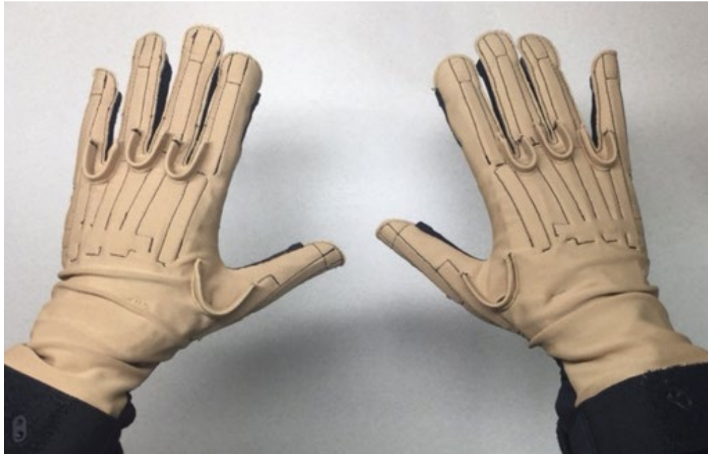
Glove attaches physical sensors to the hand.
