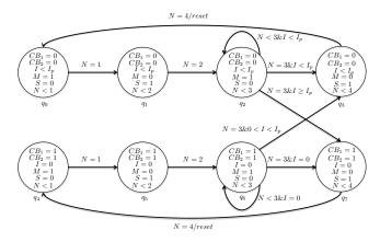
Fig. 1: Hybrid automaton for the case study
