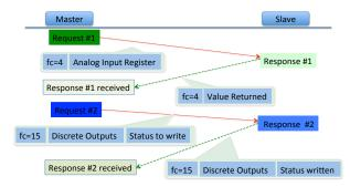
Fig. 2: Expected communication packet sequence
