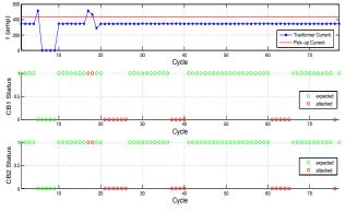
Fig. 5: Transformer's current and status of circuit breakers
