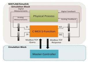
Fig. 3: Block diagram of the experimental framework
