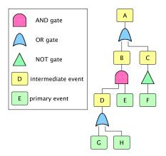
Fig. 7. Simple fault tree
