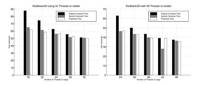
Figure 2: Redblack3D timings with 32 and 48 threads on *balder*, and varying numbers of threads on *aegir*
