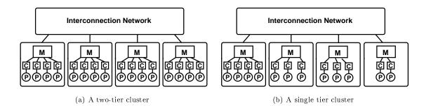
Figure 1: Block diagrams of a homogeneous (a) and homogeneous (b) dual tier clusters. M=memory, C=cache, P=processor. On-processor cache memories are not shown.
