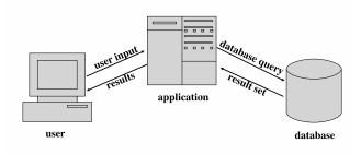
Figure 1. A typical system architecture for web applications.
