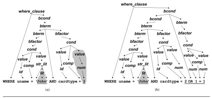
Figure 4. Parse trees for WHERE clauses of generated queries. Substrings from user input are underlined.
