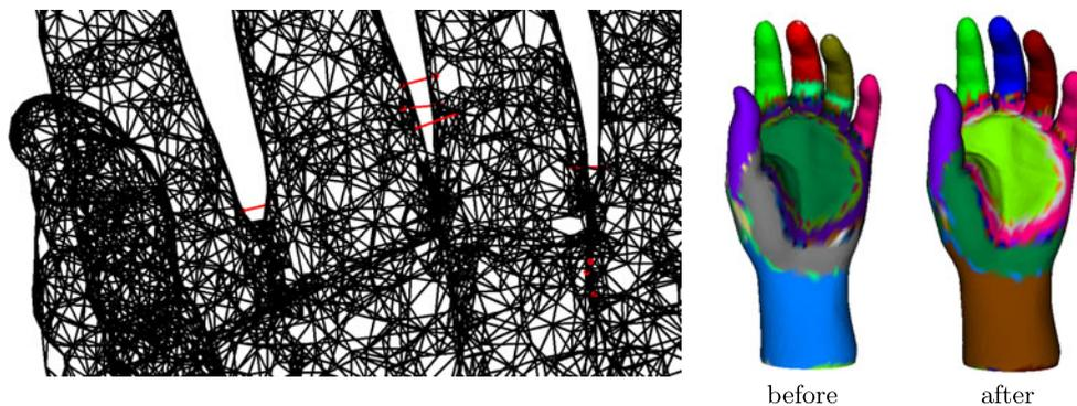
**Fig. 4** Effect of feature-crossing edges. In the left figure, the edges in red are identified as the feature-crossing edges in the  $k$ -nearest neighbor graph of the coarse model of the hand. The quality of supernodes is
