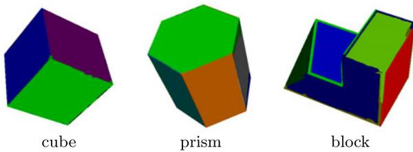
**Fig. 9** Segmentation of CAD models. Edge lengths in the  $k$ -nearest neighbor graph and in the graph of supernodes are modified before applying the multiphase segmentation process
