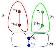
**Fig. 6** Weighted graph representing the relation of supernodes. Two vertices are created for each supernode  $s_i$ : a representative vertex  $r_i$  and a member vertex  $m_i$ . There are edges between  $r_i$  and  $m_i$ , and between  $m_i$  and  $m_j$  if and only if  $s_i$  is a supernode created at a saddle point and  $s_j$  is one of the supernodes that terminates at the saddle. In the figure,  $s_3$  is created at a saddle where  $s_1$  and  $s_2$  merge
