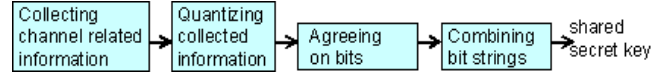
Fig. 2. Steps of generating shared secret keys in multiple-antenna systems using the channel related information.
