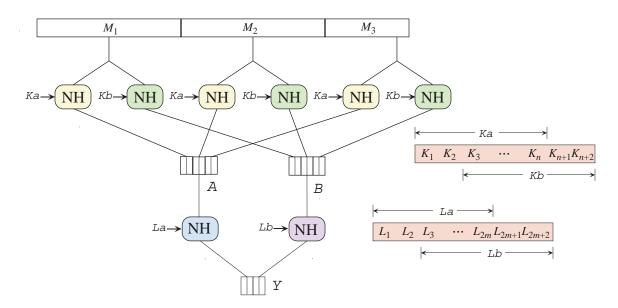
Figure 4: The T2 scheme. Each block of the message is hashed twice, first using a key Ka, and then using a key Kb. Key Kb is the shift of key Ka. The outputs of the Ka-hashes are concatenated and La hashed, and the outputs of the Kb-hashes are concatenated and then Lb hashed. Key Lb is once again the shift of key La.
