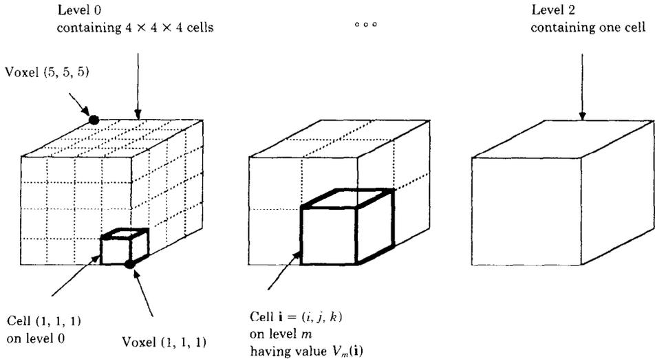
Fig. 3. Hierarchical enumeration of object space for  $N = 5$ .
