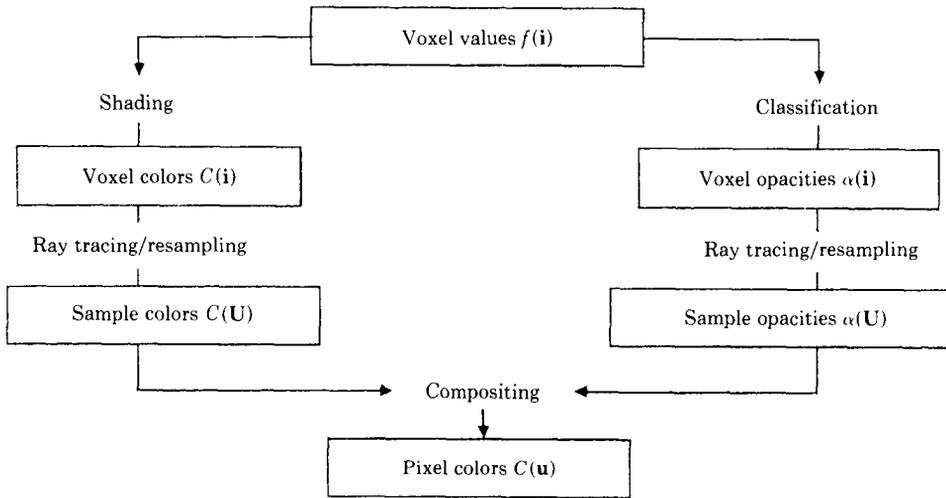
Fig. 1. Overview of volume-rendering algorithm.
