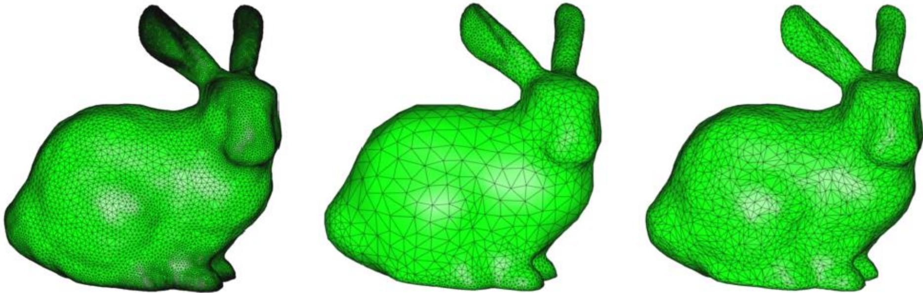
**Fig. 8.** *A comparison of our skin mesh coarsening algorithm with Qslim.*
