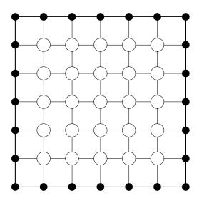
This is an example grid with N = 5. The values v(x, y) at the boundary grid points  $\bullet$  is given by  $\phi(x, y)$ , and the values v(x, y) at interior
