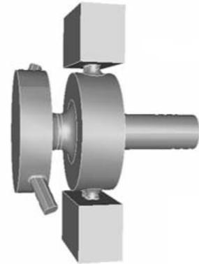
**Figure 3.** Omega3P model of the Linac Coherent Light Source radiofrequency cavity. Courtesy of the Advanced Computation Department, SLAC.
