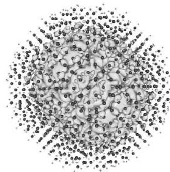
**Figure 1.** Isosurface rendering of an eigenvector associated with an eigenvalue in the conducting band of a silicon quantum dot. The larger and darker balls in the figure correspond to silicon atoms. The smaller and lighter balls correspond to hydrogen atoms. Image courtesy of Lin-wang Wang of LBNL.
