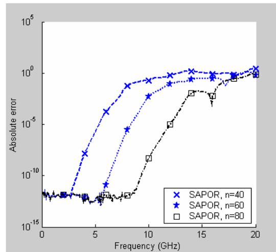
Figure 4. Errors of SAPOR with three different orders
