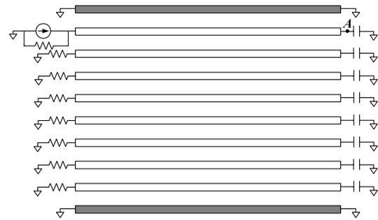
Figure 2. 8-bit bus with two shielding lines
