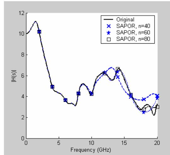
Figure 3. Comparison of frequency responses by SAPOR with three different orders
