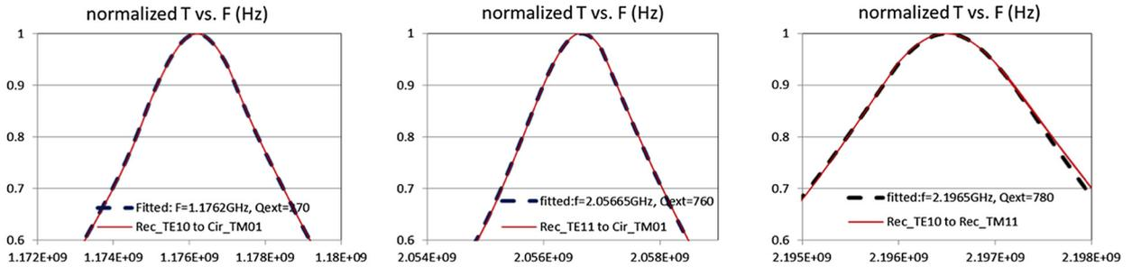
**Fig. 3.** Normalized transmission curves and the Lorentzian fit for the cavity modes at 1.176 GHz (left), 2.057 GHz (middle), and 2.196 GHz (right).
