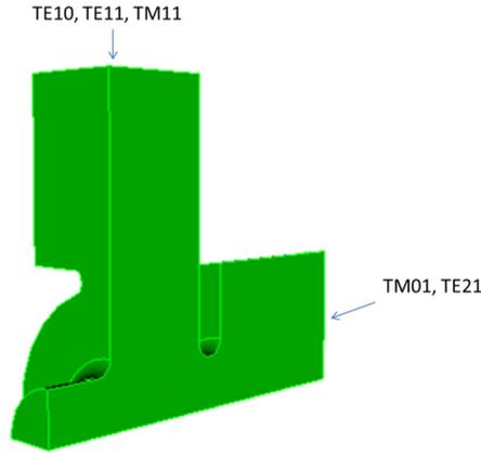
**Fig. 1.** A quarter model of a pillbox cavity coupled with rectangular waveguides and circular beampipes. The two symmetry planes are set to be magnetic boundary conditions. Three rectangular and two circular modes are loaded at the rectangular and downstream circular waveguides, respectively.
