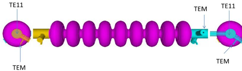
**Fig. 4.** TESLA cavity with one fundamental power coupler (FPC) and two higher-order-mode (HOM) couplers. The FPC and HOM couplers are loaded with a coax TEM mode and the two beampipe ends are loaded with two polarizations of the circular TE11 modes.
