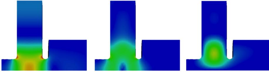
**Fig. 2.** Electric field amplitude profiles on the vertical symmetry plane for cavity modes at 1.176 GHz (left), 2.057 GHz (middle), and 2.196 GHz (right).
