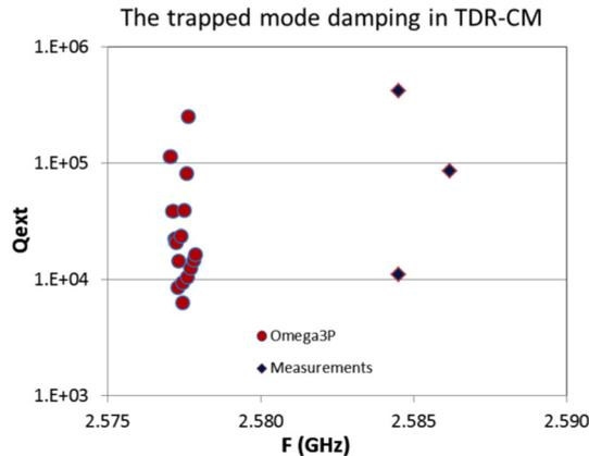
**Fig. 5.** Comparison of trapped mode damping calculations in an ideal LCLS-II 8-cavity cryomodule using the CORK nonlinear eigensolver in Omega3P and experimental measurements. The simulated frequencies are shifted for about 10 MHz to lower values due to cavity imperfection.
