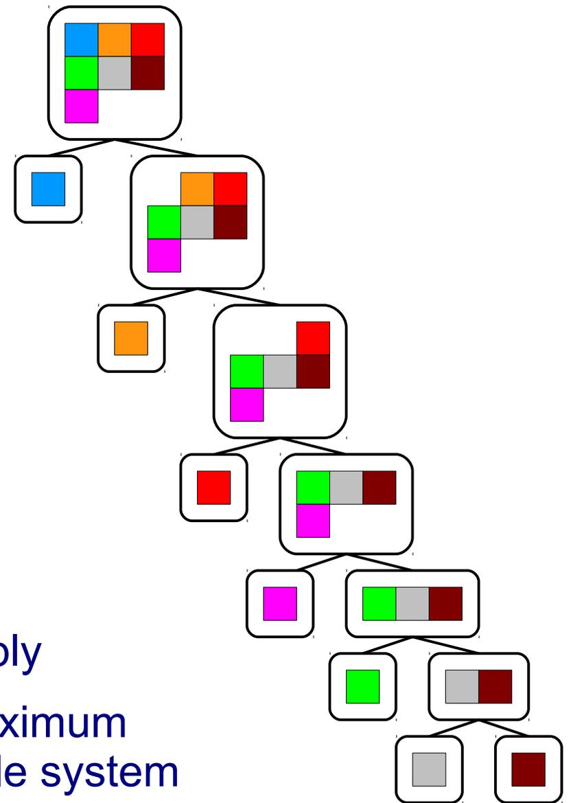
assembly tree = possible order of attachments leading to final assembly
