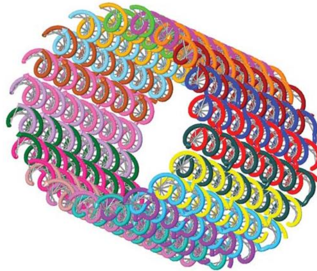
DNA-level diagram of 20-helix tube
