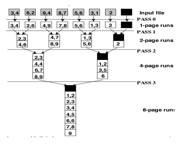
• 2-way merge sort can be generalized to *n*-way merge sort, using as many interal buffer pages as we have available
