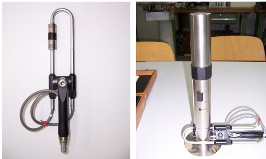
Fig. 6. The sound intensity probe and the calibrator.
