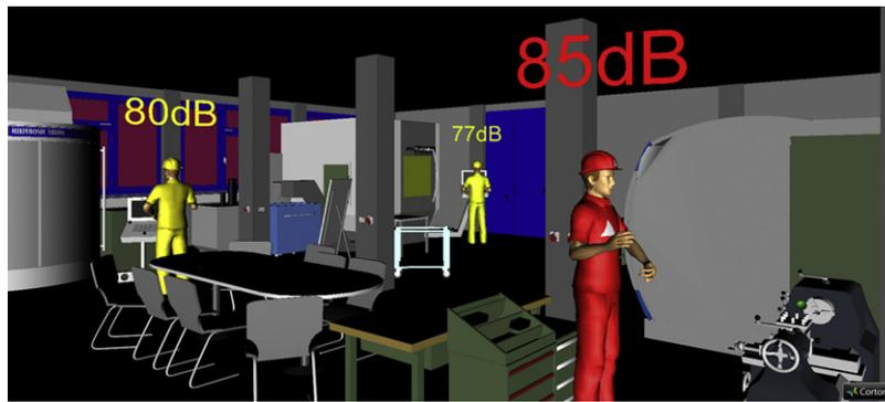
Fig. 16. Visualization of sound pressure level at different positions.
