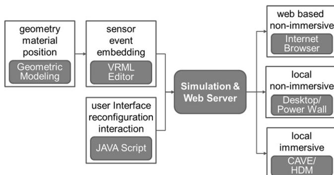
Fig. 11. The VRML supported software framework.
