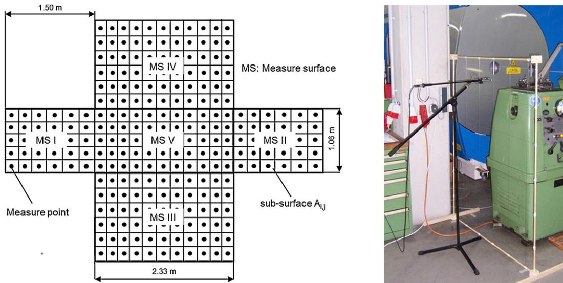
Fig. 5. Sound power measurement blue print and support equipment.
