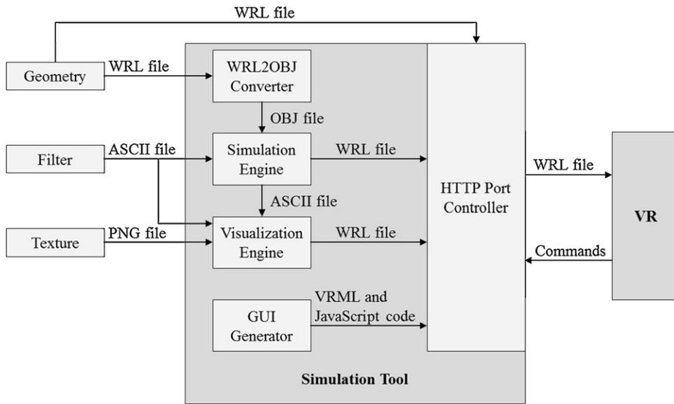
Fig. 12. Function diagram of simulation and visualization software tool.
