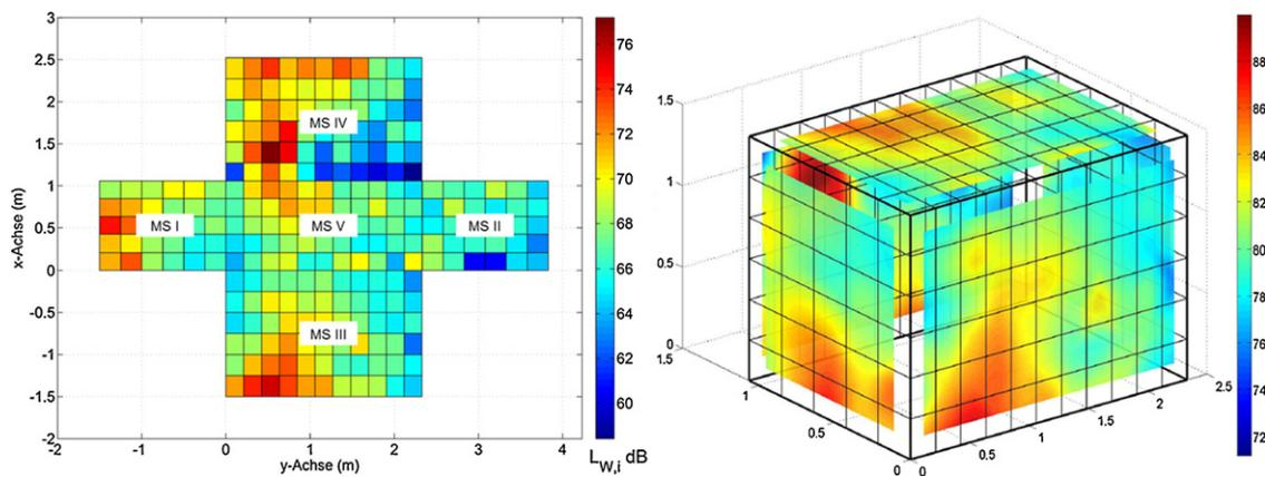
Fig. 7. Visualized sound power level in 2D and 3D.
