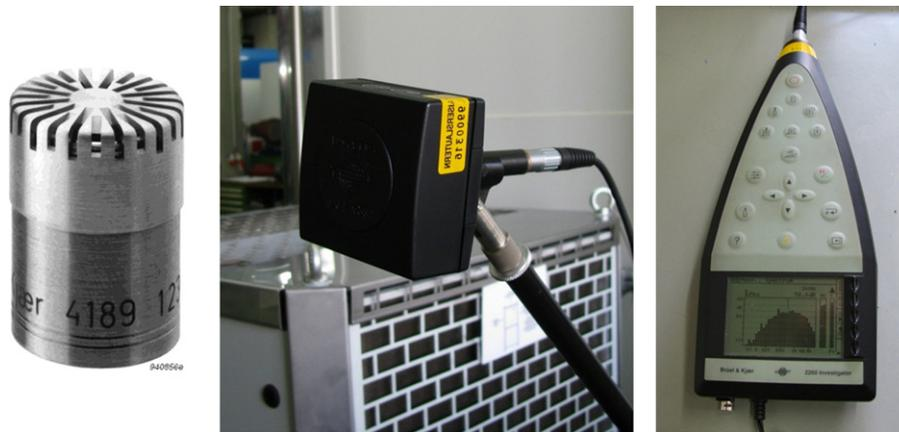
Fig. 8. Microphone, calibrator and measurement setting.
