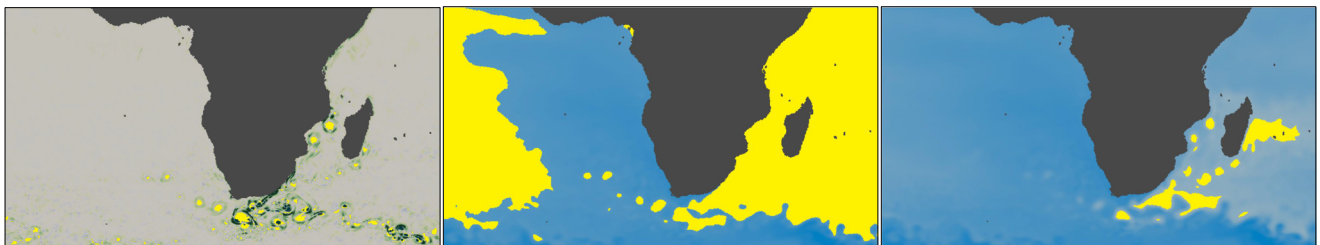
Fig. 23 Simulation-derived features for Eddy detection. To identify eddies in Agulhas region using sea surface height in Paraview, two sets of thresholds must be selected to capture the entirety of the eddies. However, only a single threshold range is needed when evaluating Okubo-Weiss
