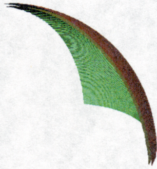
Figure 7: Boundary surfaces of two materials formed as two concentric spherical “shells”.
