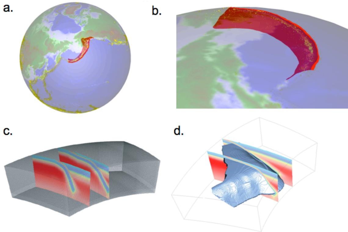
Figure 3. Constructing, viewing, and refining a model of a slab (adapted from the work of Jadamec and Billen 2006). (a) Global earthquake distribution in a transparent globe. (b) Slab surface constructed from seismic data (see text for references). (c) Arbitrary slices taken through a finite element model of a slab using the slicer tool. (d) Seeded isosurface with slices.
