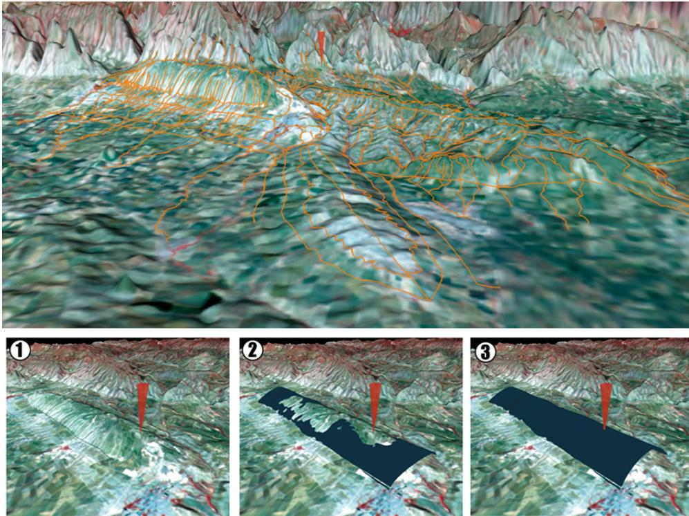
Figure 2. Top: Using the 3D view of RIMS with a twofold vertically exaggerated textured DEM, structures were more easily identified and could be directly mapped out. Bottom: Interpreting the 3D geometry of a surface (a fold). Modified after Bernardin et al. (2006)
