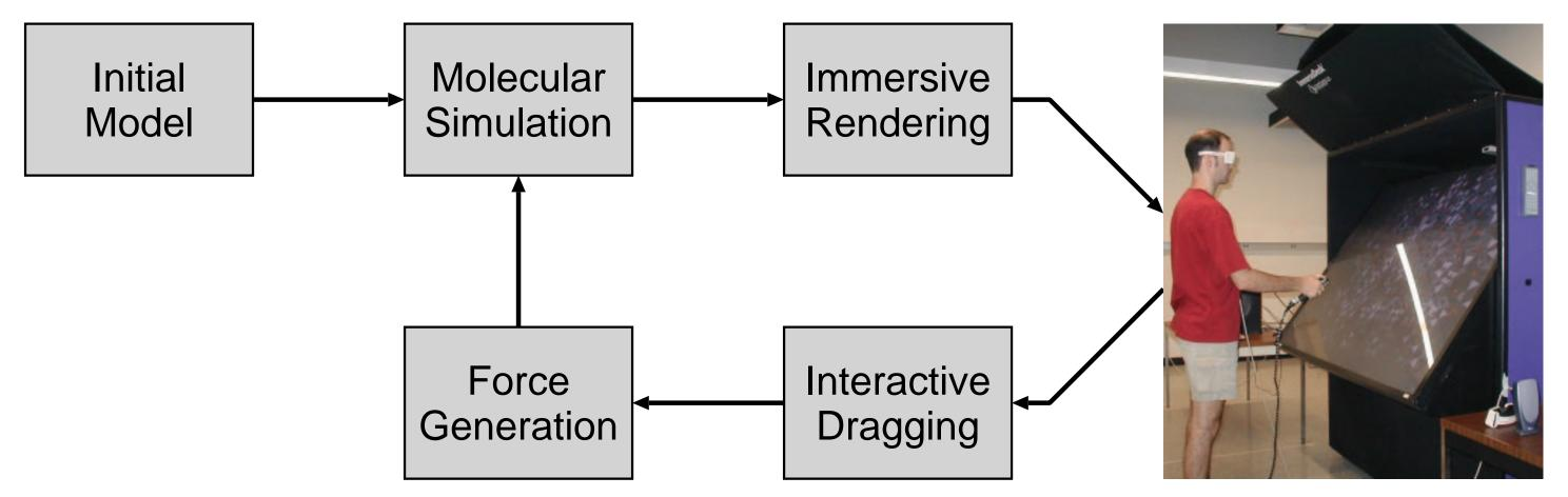
**Figure 1:** Diagram of the feedback loop of an interactive simulation system. The user is integrated into the loop using head-tracked stereoscopic display and six-degree-of-freedom input devices.
