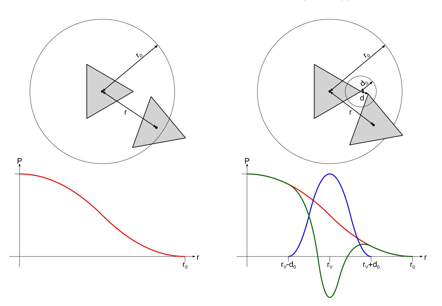
**Figure 2:** Diagram of the potential £eld used in the Nanotech Construction Kit. Left: Interaction between two non-bonded units (red: repulsion potential). Right: Interaction between two bonded units (red: repulsion potential, blue: bond attraction potential, green: result potential).
