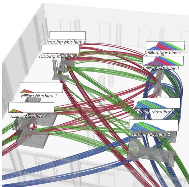
**Fig. 1** Flow view of a virtual production system showing the geometric model of the factory and its machines, the product flow for all products color-coded by product type, and the machine workloads for all machines
