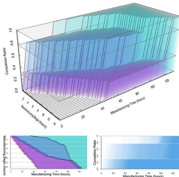
**Fig. 6** Production view for all products of type C showing inactive and processing phases of their three operations under different aspects of manufacturing time, manufacturing begin, and degree of completion
