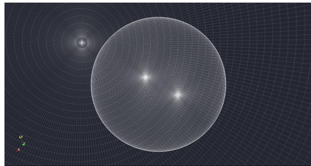
Figure 3: Depiction of the cell structure of the underlying data. An unstructured grid is used for the description. The size of the cells vary with increasing radius. As well when going from top to bottom. In itself the structure is regular, which means the size changes linear with the components (in spherical coordinates) and finer in radial direction near the boundaries. The dataset covers only a shell of a sphere, because the inner core is excluded from the simulation.
