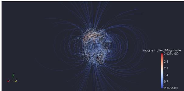
Figure 2: Streamline visualization using an extended domain, containing the simulation domain of the outer core and a potential field for the magnetic field outside the simulation domain. Using 100 seed points placed in sphere around the center for streamline tracing. Showing of the dipole structure of the magnetic field as also known from physical experiments.
