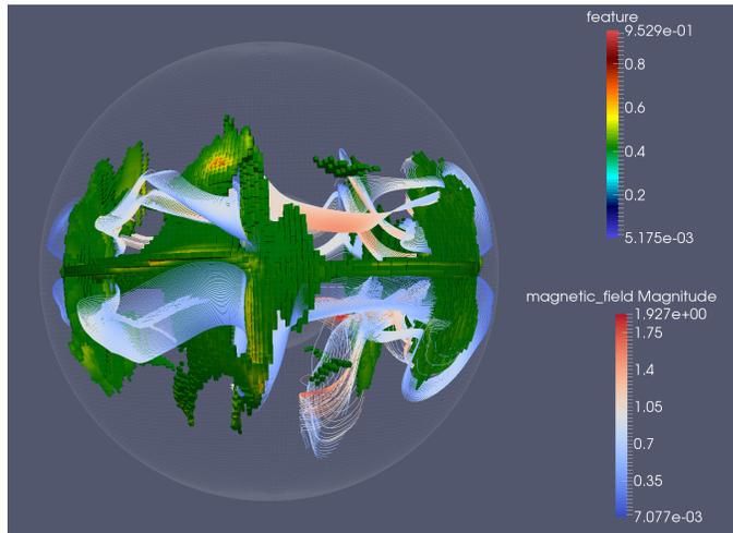
Figure 5: Full sized visualization of the magnetic field using ADCR for seeding in all topological relevant areas including ADCR visualization using threshold volume. View from equator.
