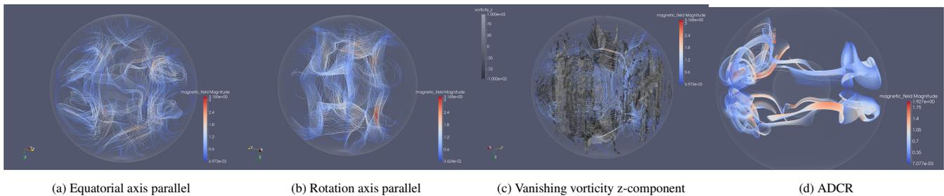
Figure 6: Comparing different strategies for seeding streamlines to visualize the magnetic field. All seeding is done by a high resolution line source. Fig. 6a and Fig. 6b using regularly spaced lines parallel to the respective axis in the middle of the domain. Fig. 6c generated by placing the lines inside the vanishing z-component areas. Fig. 6d seeding in high turbulent areas and in encapsulated low turbulent areas (wholes in Fig. 5).
