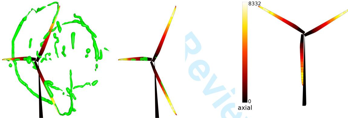
(a) Extracted vortices and turbine. (b) Intersections of vortices and turbine geometry.
