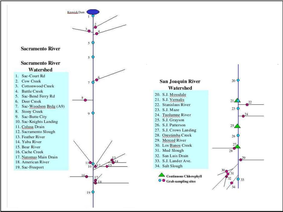
**Figure 2.** Schematic layout of monitoring stations on *left*: Sacramento River and *right*: San Joaquin River. (Image courtesy of U.S.Bureau of Reclamation)
