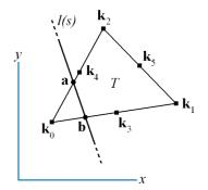
**Figure 3:** Intersection of line l(s) with linear-edge quadratic triangle T(u, v) at points **a** and **b**.
