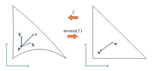
**Figure 5:** Inverse transformation of vector  $\mathbf{v}$ —located at point  $\mathbf{p} = T(\mathbf{u})$ —through curved-quadratic mapping T(u, v). Vector  $\mathbf{v}$  is transformed from physical space to vector  $\mathbf{w}$  in parameter space by considering the linear combination  $\mathbf{v} = \alpha \mathbf{X} + \beta \mathbf{Y}$ , where  $\mathbf{w} = (\alpha, \beta)^{\mathrm{T}}$ .
