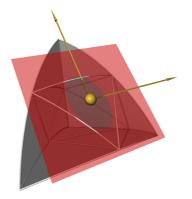
**Figure 10:** Intersection of plane and curved-quadratic tetrahedron. Difficulties arise since the plane can intersect the tetrahedron without intersecting its edges. (In this paper, quadratic tetrahedra are often rendered with parametric lines on the faces of the element. These lines help show the curvature of the element. Plane R intersects the parametric lines shown on the faces of tetrahedron T, however, these lines are not as useful as the edges of the tetrahedron.)
