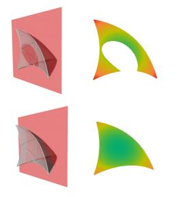
**Figure 12:** *Two cutting planes intersecting curved-quadratic tetrahedron.*
