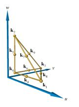
Figure 9: Indexing used for curved-quadratic tetrahedron.
