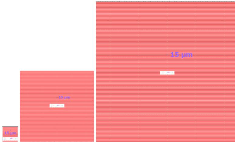
Fig. 3. Retina motion traces from Fig. 2 scaled to the 1x1mm, 5x5mm and 10x10mm areas used to acquire AO-OCT and OCT data sets. The OCT beam spot of 15μm is shown for comparison.
