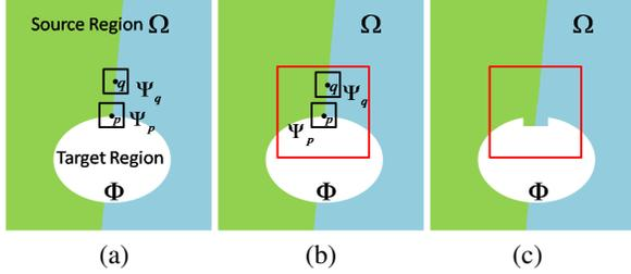
**Fig. 1.** Basic notions of image inpainting method.
