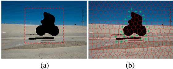
**Fig. 3.** (a) Original image with black hole; (b) Superpixel segmented image. Superpixels marked with green stars are used for inpainting.
