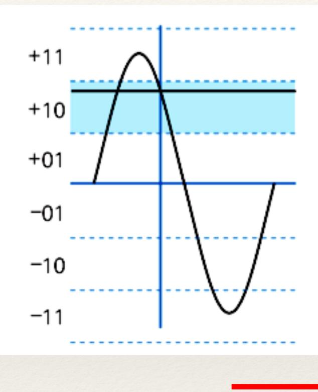
Adding one bit makes the sample twice as accurate
