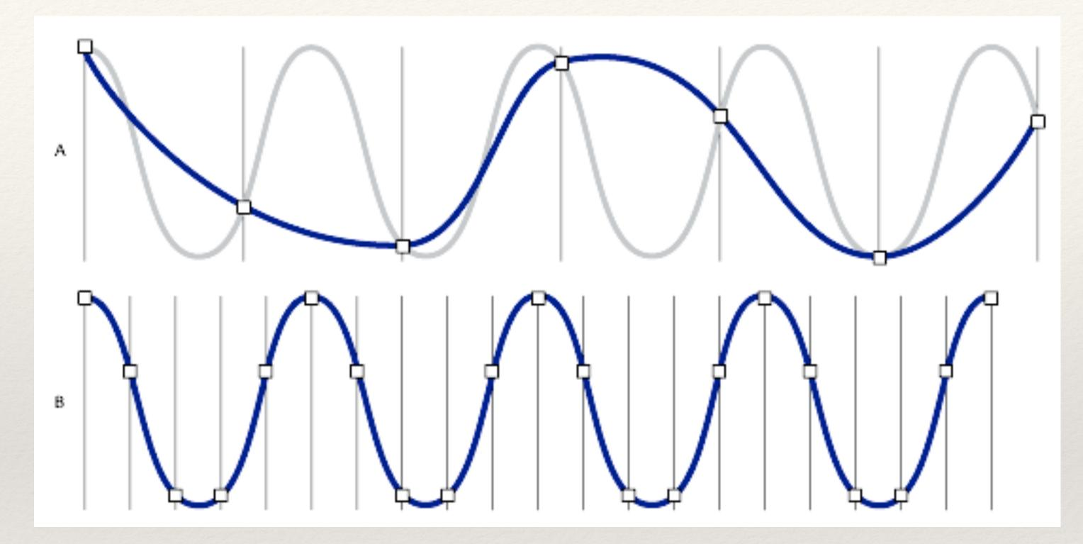
A higher sampling rate usually allows for a better representation of the original sound wave. However, when the sampling rate is set to twice the highest frequency in the signal, the original sound wave can be reconstructed without loss from the samples. This is known as the Nyquist theorem.
