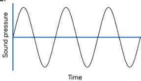
To store and process sound information in a computer or to transmit it through a computer network, we must first convert the analog signal to **digital form** using an analog-to-digital converter ( ADC ); the conversion involves two steps: (1) **sampling**, and (2) **quantization**.
