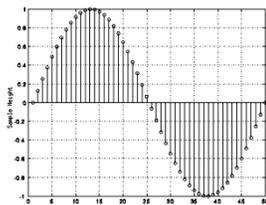
Sampling usually occurs at **uniform** intervals, which are referred to as **sampling intervals**. The **reciprocal** of sampling interval is referred to as the **sampling frequency** or **sampling rate**. If the sampling is done in **time domain**, the unit of sampling interval is **second** and the unit of sampling rate is **Hz**, which means **cycles per second**.
