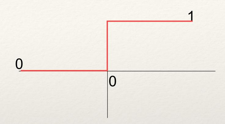
The output F is a function of S: it is often set discrete (i.e. 1 or 0), in which case the function is the step function.
