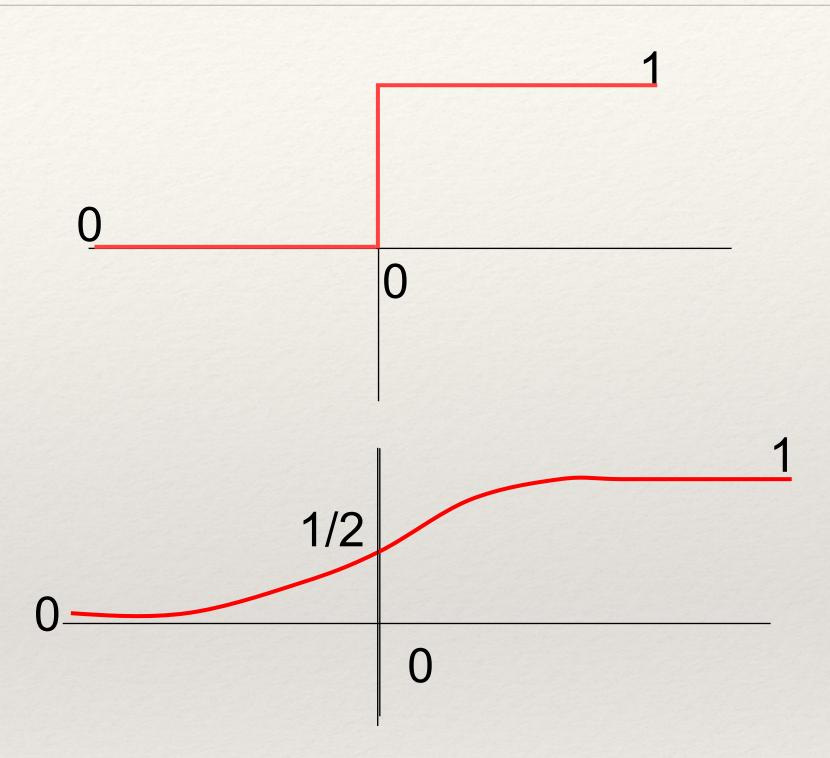
The output F is a function of S: it is often set discrete (i.e. 1 or 0), in which case the function is the step function.
