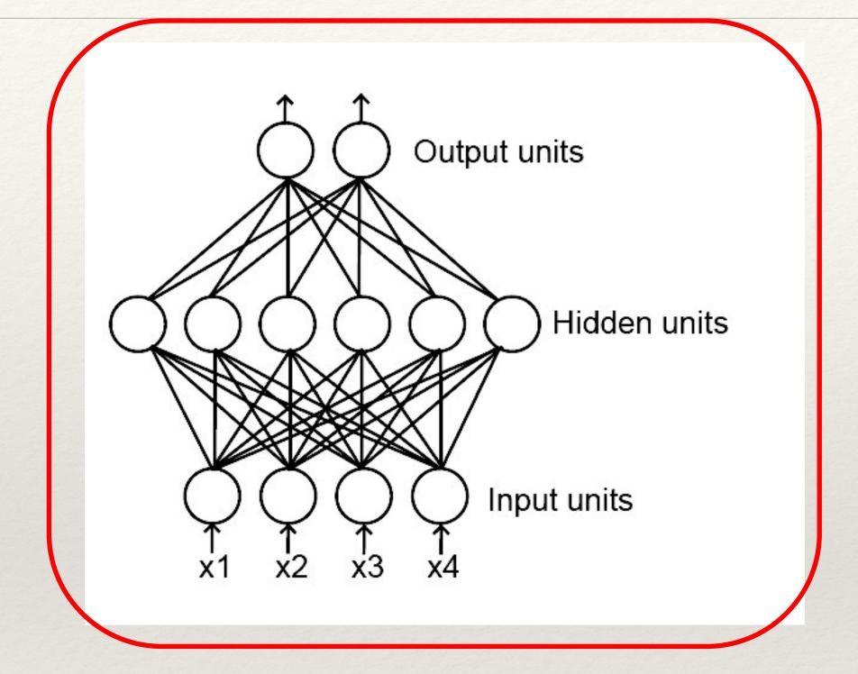
A complete neural network is a set of perceptrons interconnected such that the outputs of some units becomes the inputs of other units. Many topologies are possible!
