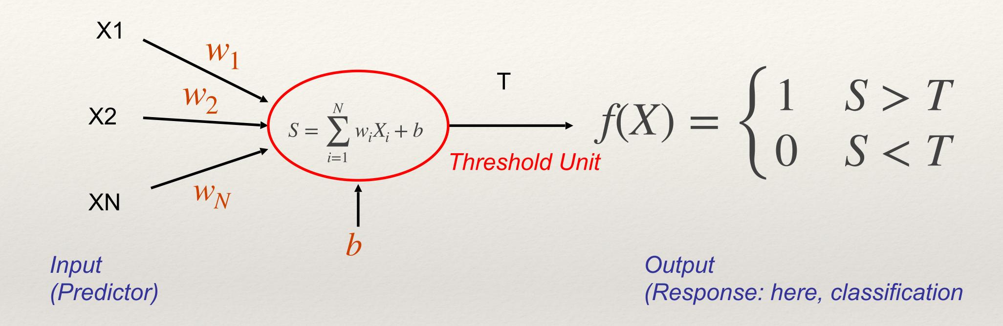
If the weights, bias, and threshold T are not known in advance, the perceptron must be trained. Ideally, the perceptron must be trained to return the correct answer on all training examples, and perform well on examples it has never seen.
