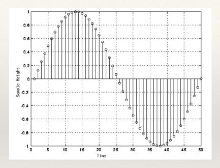
Sampling usually occurs at uniform intervals, which are referred to as sampling intervals. The reciprocal of sampling interval is referred to as the sampling frequency or sampling rate.
