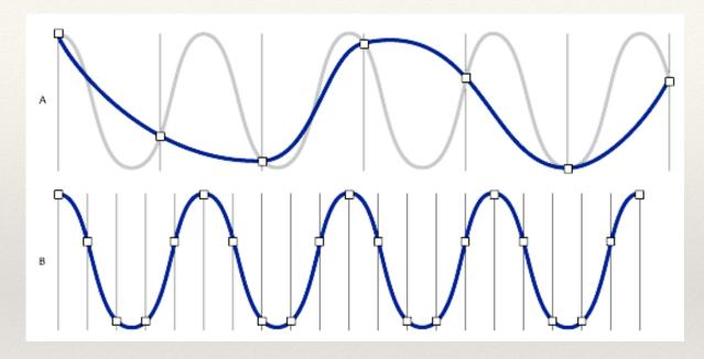
A higher sampling rate usually allows for a better representation of the original sound wave. However, when the sampling rate is set to be strictly greater than twice the highest frequency in the signal, the original sound wave can be reconstructed without loss from the samples. This is known as the Nyquist theorem.
