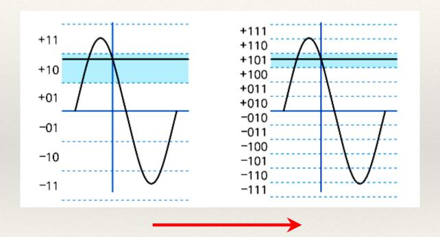
Adding one bit makes the sample twice as accurate
