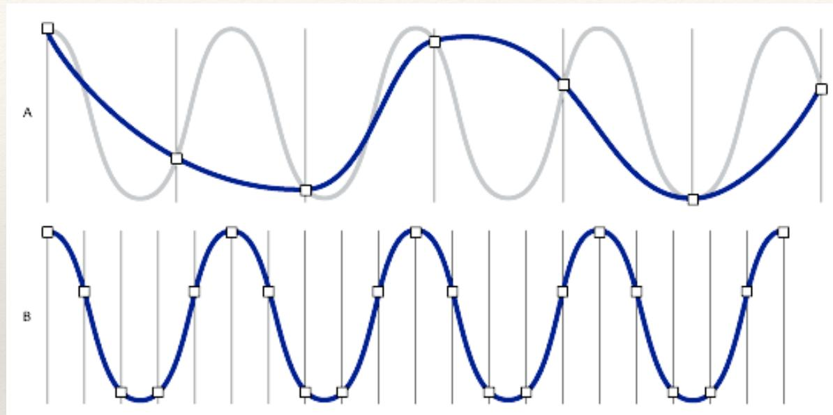
A **higher** sampling rate usually allows for a **better** representation of the original sound wave. However, when the sampling rate is set to be **strictly greater than** twice the highest frequency in the signal, the original sound wave can be reconstructed without loss from the samples. This is known as the **Nyquist theorem**.
