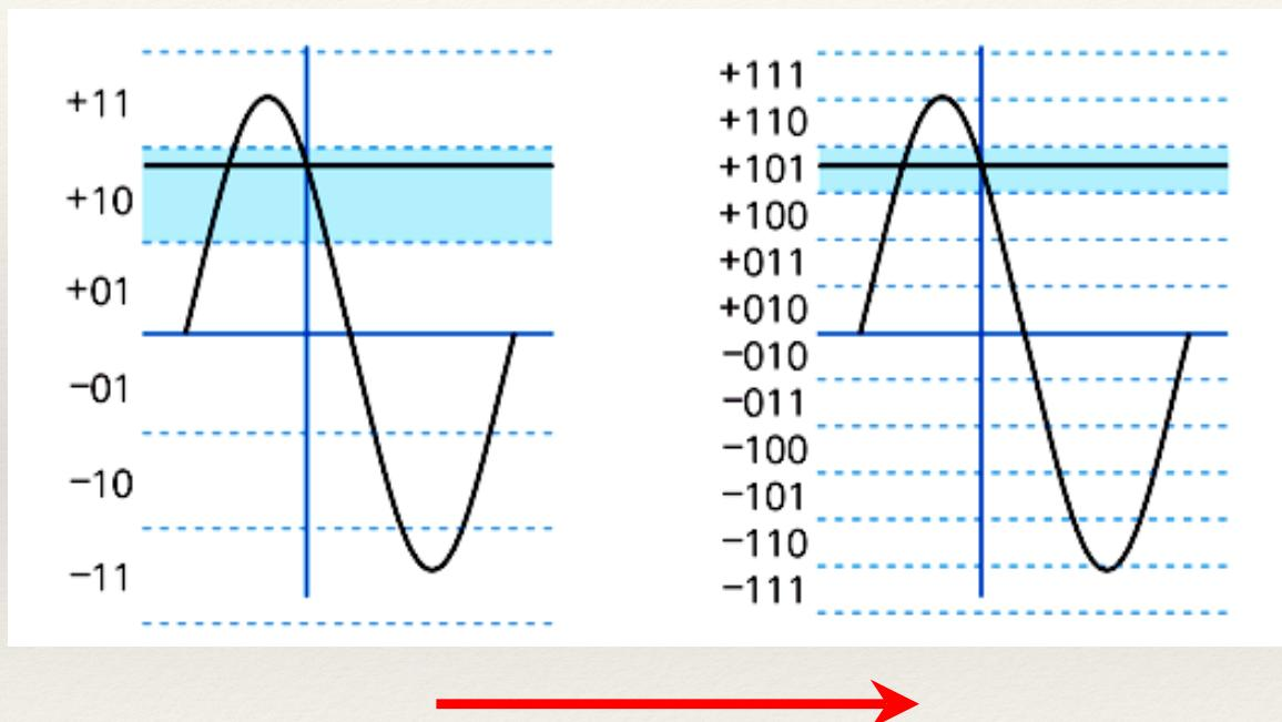
*Adding one bit makes the sample twice as accurate*
