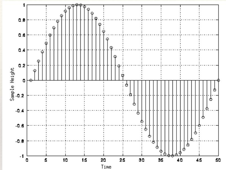
Sampling usually occurs at **uniform** intervals, which are referred to as **sampling intervals**. The **reciprocal** of sampling interval is referred to as the **sampling frequency** or **sampling rate**.
