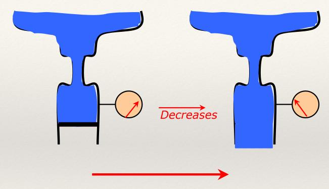
When we remove the block, what is the effect on pressure?
