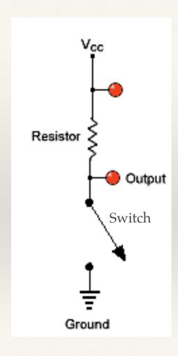
If switch is off (0) (equivalent to the presence of the block)
