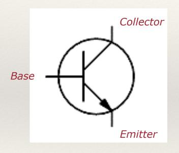
A transistor can be used as an electronic switch:
