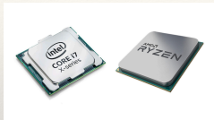
CPUs are getting smaller, and can include more than one "core" (or processors).
