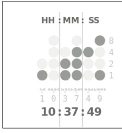
Add the values of each column to get six decimal digits. There are two columns each for hours, minutes and seconds.
