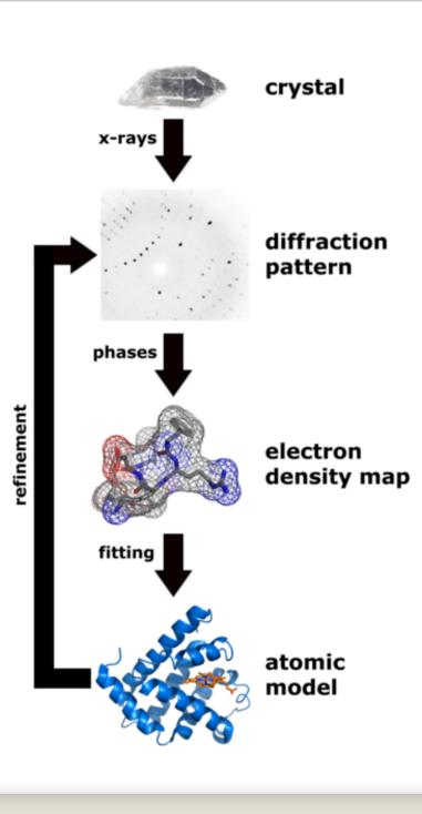
General principle of X-ray crystallography applied to proteins:
