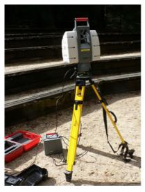
C) Laser scanner: triangulation
