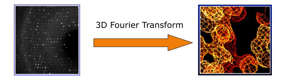
**One hidden problem:** diffraction patterns provide intensities; for Fourier transform, need intensity and phase. A significant step in X-ray crystallography is the solve the "phase problem".
