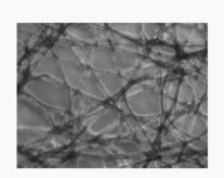
Bright field illumination, sample contrast comes from absorbance of light in the sample. Cross-polarized light illumination, sample contrast comes from rotation of polarized light through the sample. Dark field illumination, sample contrast comes from light scattered by the sample.
