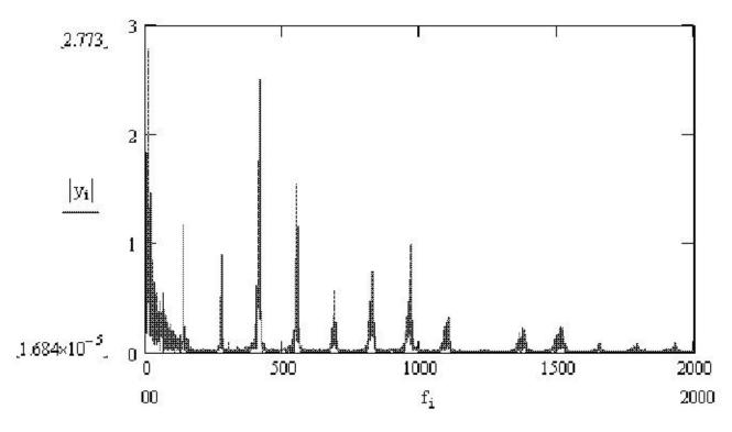
Note that this graph is very "spiky." In other words, most of the power of the signal is at a few frequencies which arise from the physical properties of a reed.
